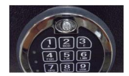
Carefully remove the keypad cover from the housing. Let the keypad cover hang with the wires still attached
