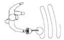
It is better you sweep the search coil from side to side in an arc line of 3 inches motion and keep the search coil parallel with the ground.
