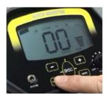
Press NOTCH again and the selected target ID will disappear. It means that this target will be notched during the detection, and the detector will
