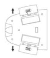
You need two 9V alkaline batteries to power your detector.
