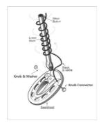
3. Loosen the middle stem's lock nut in the direction of the arrow. Then, insert the lower stem into the middle stem. Turn the stem's lock nut in the reverse direction of the arrow to lock it in place.
