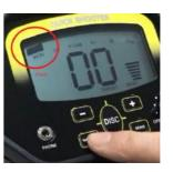
a. Press NOTCH and then press + or - to select the Target Indicator to be notched. The cursor above the selected target will flash.
