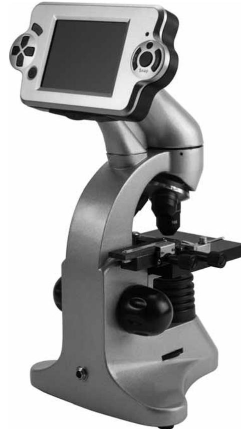
16x, 40x, 160x Magnification with LCD screen
