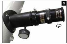
Choose one (B) eyepiece and insert the Barlow Lens of the eyepiece into the (L) Barlow and tighten the set screw.
