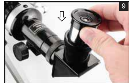
9 Choose one (B) eyepiece and insert the chrome barrel of the eyepiece into the (C) diagonal and tighten the set screw.
