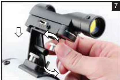
7 Remove the (K) knurled nuts and attach the (I) finderscope to (L) main telescope optical tube with the battery compartment and lens facing the front of the telescope. Secure by tightening the (K) knurled nuts.
